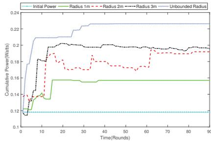
Fig. 5. The cumulative system power during a random execution of the first algorithm for different communication ranges of the chargers.
