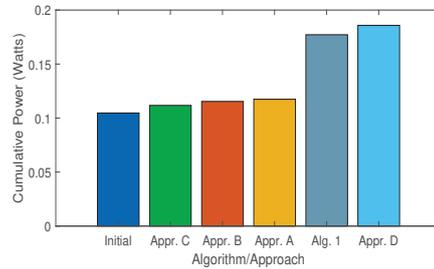
Fig. 10. Mean cumulative device power after executing each approach for 100 different network topologies, with movement area radius equal to  $\lambda/2$  for every algorithm.
