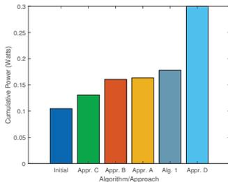
Fig. 7. Mean cumulative device power after executing each approach for 100 different network topologies.
