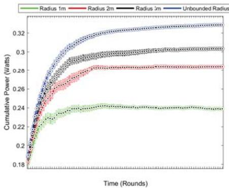
Fig. 6. Confidence intervals for the mean of the cumulative power of the devices for different communication ranges during 100 executions of the first algorithm.
