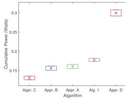
Fig. 8. Confidence intervals for the mean of the cumulative device power after executing each approach for 100 different network topologies.
