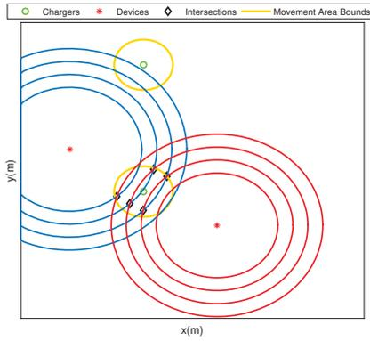
Fig. 4. Simple example with two chargers and two devices, showing the intersections between the sets of circles for the two devices. If the charger is set at any of the intersection points, both devices will be on a superadditive interference point.
