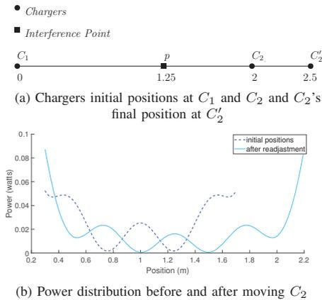
Fig. 2. Example with two chargers  $C_1$  and  $C_2$ , showing that moving  $C_2$  away from some points, to the point  $C_2'$ , can increase their received power. The point  $p$  is one of them.
