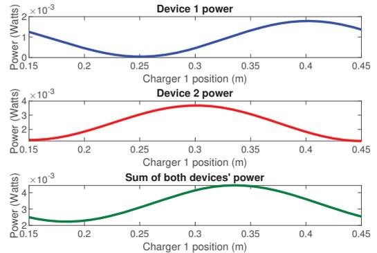
Fig. 3. Example showing the power of two devices when moving one charger.
