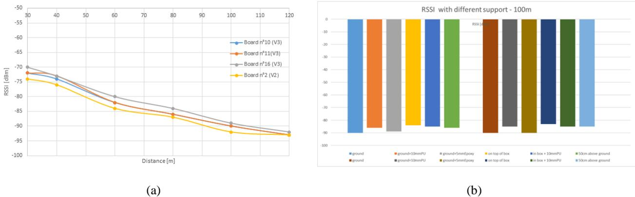
Fig. 4 (a) Ranging measurement of BLE channel during the 2<sup>nd</sup> testing iteration. The ORUs were placed on the road surface while the RSB is installed on the building (8 meters above the ground), (b) RSSI of the BLE packets placing the ORU at different heights from the ground.
