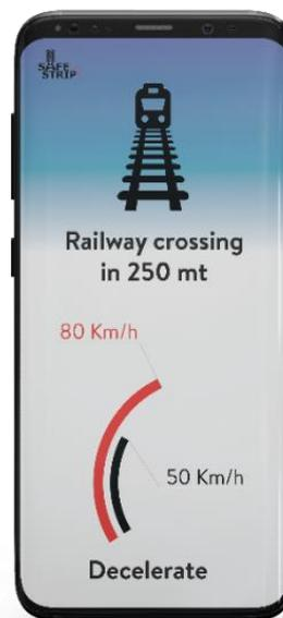
Fig. 2. HMI mobile application early prototype
