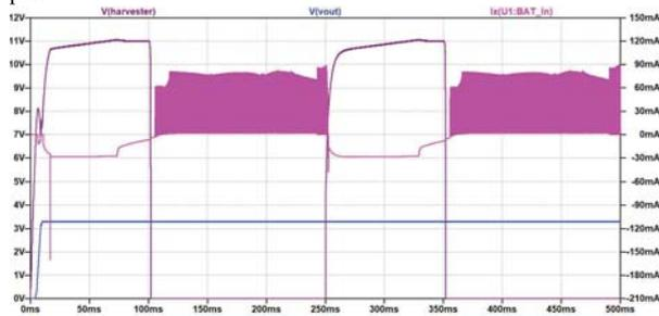
(c) Harvester and output voltage and current flowing through  $BAT\_IN$  pin.
