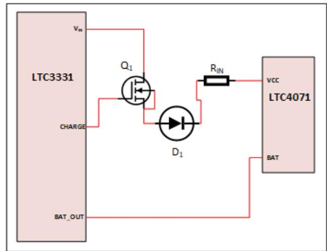
Fig. 4: LTC3331 combined with LTC4071 to allow more charging current to the rechargeable batteries.
