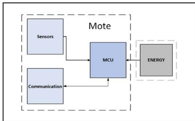
Fig. 1: High level schematic of a mote including sensors, MCU and communication. The connection with the energy part is also depicted.
