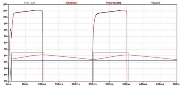
(a) Harvester, battery, output voltage and  $EH\_ON$  signal.
