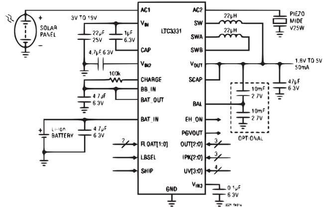
Fig. 3: Typical application of the LTC3331 ([13]) using a solar panel and a piezo energy harvester to provide 1.8 to 5V to the output and charge a single cell Li-Ion battery.
